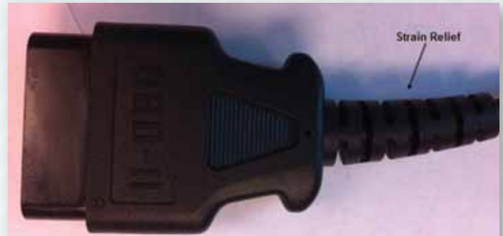
Figure 4, Lengthened Strain Relief on OBD-II Cable
