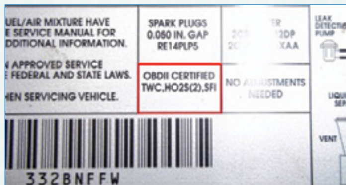
This VECI label indicates that the vehicle was not manufactured with an EGR system monitor.
