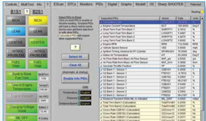
Looking at scan tool oxygen sensor values (in the blue box) doesn't always reveal what needs to be repaired.
