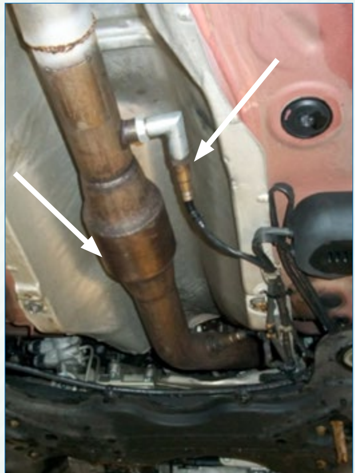
Catalytic converter and oxygen sensor tampering are indicated by the white arrows above.
