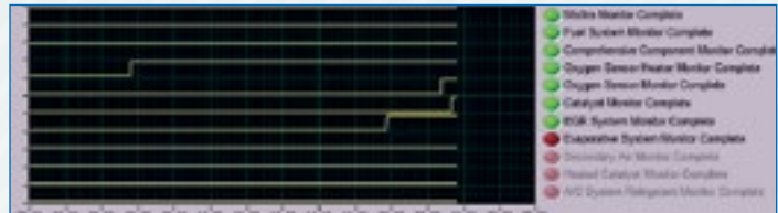
After the torn air boot was replaced, the Mazda Protégé reset all but one of its OBD monitors within 23 minutes.
