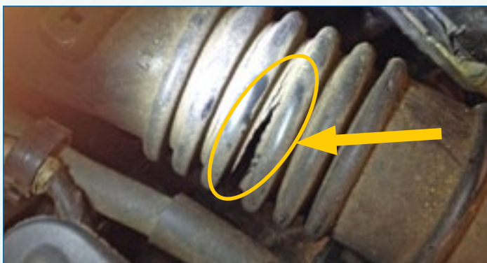
When the Tewksbury MAC L1 performed a simple visual inspection, he discovered a torn air boot between the MAF and the throttle body.
