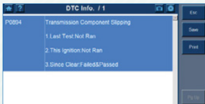
The 2003 GMC Safari had a historical P0894 Transmission-Related Diagnostic Trouble Code stored in PCM memory.
